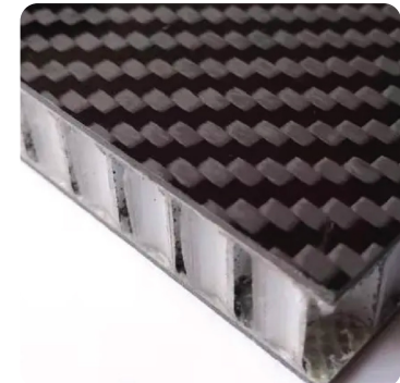
Honeycomb Fibreglass Floor
